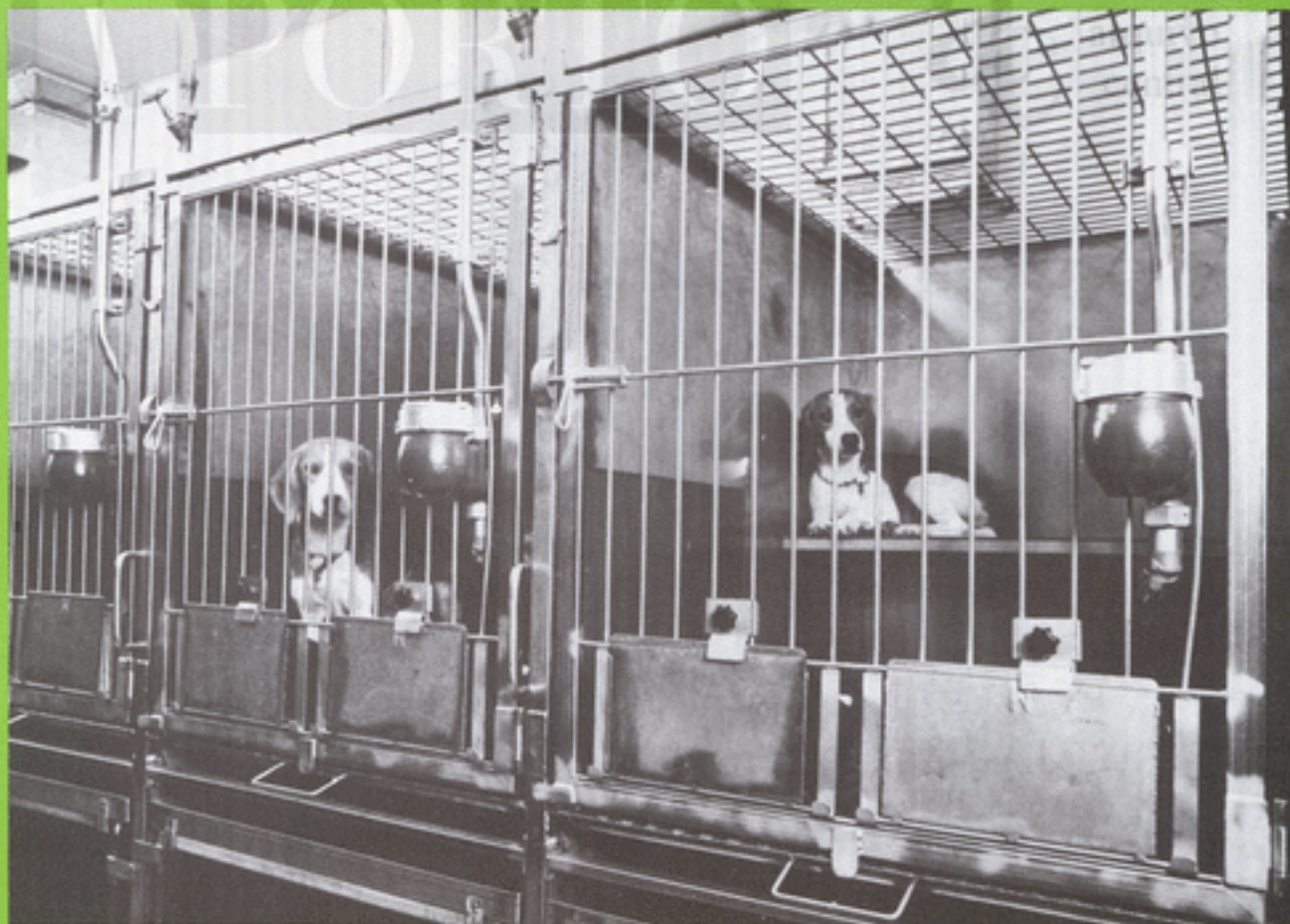
Units for single and group keeping in boxes with devices for metabolic experiments
